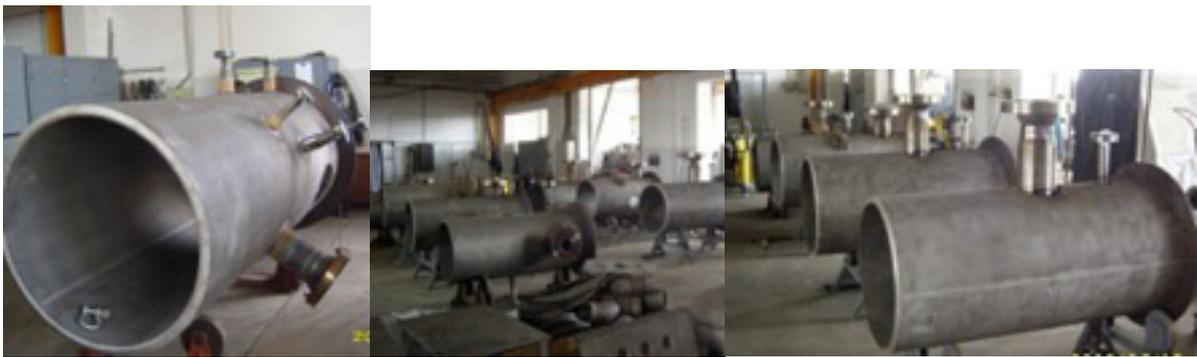
**Project Rosneft Propane/Propylene Plant:** Gas coolers (Shell and Tube 3,5MW Capacity each)
